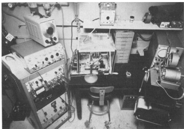
FIG. 12. Multiple chamber system, wide-angle view showing all of the components of the system as used. The electronic signal source and detection equipment is on the left. In the upper left, AC and DC signal sources are on top of a moveable panel-mount rack. The rack contains, in order from the top: the Bak electrometer amplifier; the thermistor thermometer gauge and electronic switching unit; a device for plating Ag/AgCl electrodes; a function generator which can serve as a sine, triangular, or square wave signal source; the AC amplifier, rectifier, and DC driver amplifier for strip chart recording; and the power supply for the Bak amplifier. The seated investigator can operate all equipment, observe the membrane, and collect all necessary data. The photomicroscope is in front of the membrane chamber assembly and other equipment shown in Fig. 11. The light source is directly under the photomicroscope and hidden by it. White micrometer syringes are mounted on either side of the screen cage just above the table. Above the screen cage, on the shelf, is the peristaltic perfusion pump. Visual observation, electrical data, and event marks are recorded on the right. The oscilloscope is in the upper right with its recording camera in right center. The strip chart recorder with event markers is positioned so that notes may be made directly on the chart while recording. The thermoregulated bath is on the floor at right.
